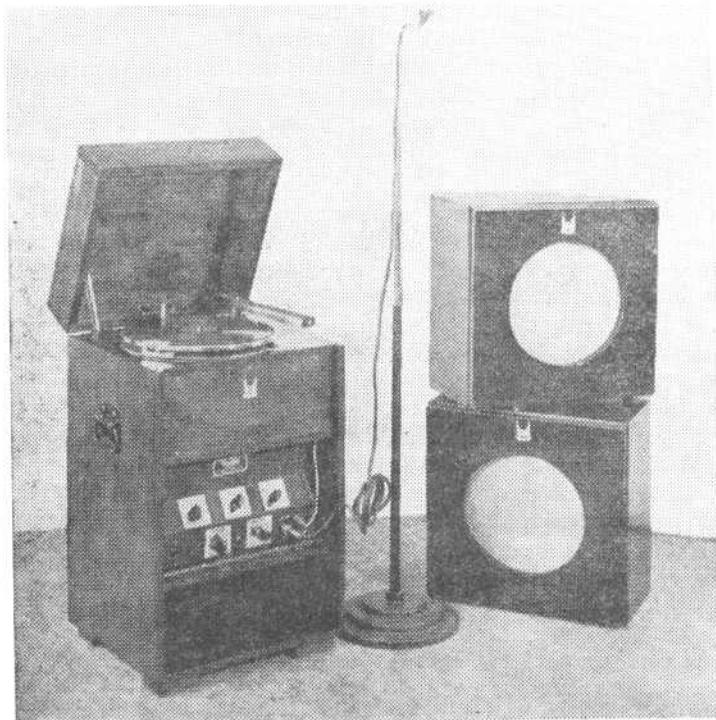
Healing portable amplifier unit for assembly, rhythm, physical culture instruction, sports, etc., with microphone and "mixing" control for recorded music and voice.
