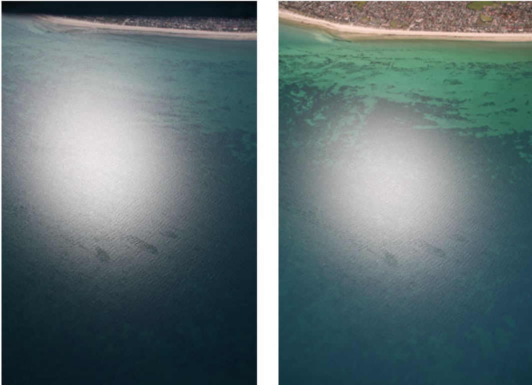
Figure 44 Frames 0754 (horizontal polarisation left) and 4735 (vertical polarisation right) - approaching coast with full sun reflection. Top of frame to the east.
