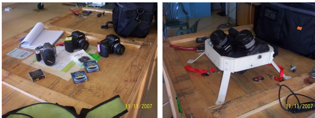
Figure 34 – Two Canon EOS 5D cameras and mounting bracket. Note the slimmer body Canon 350D camera on the left for comparison.
