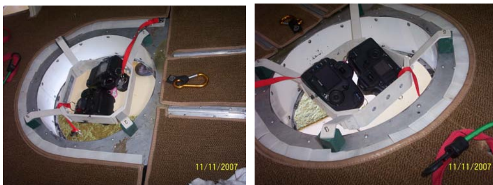
Figure 35 - Interior view of camera port and camera bracket (with cameras mounted).
