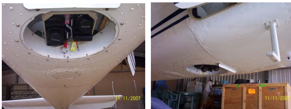
Figure 36 - Camera mounted 30 degrees forward from nadir.
