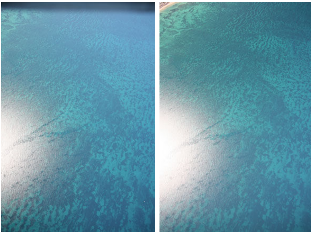
Figure 42 Comparison of horizontally polarised (frame 0613 left) and vertically polarised (frame 4594 right). Note the improvement in contrast of benthic detail top right of the frame 4594. Top of frame towards south-east.
