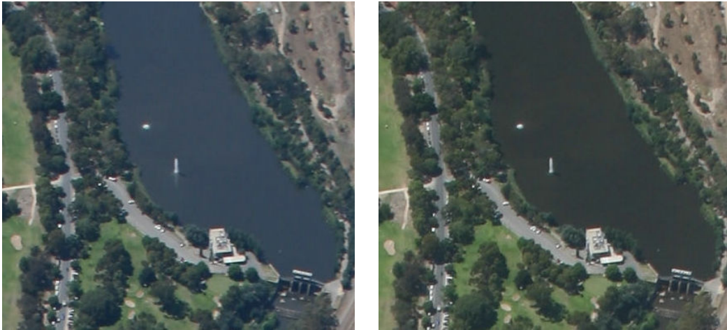
Figure 51 Enlargement of frame 0763 (horizontal polarisation left) and frame 4744 (vertical polarisation right) at the Torrens weir in the Adelaide parklands. Note the blue sky reflectance on frame 0763 and the visible brown turbidity on frame 4744.
