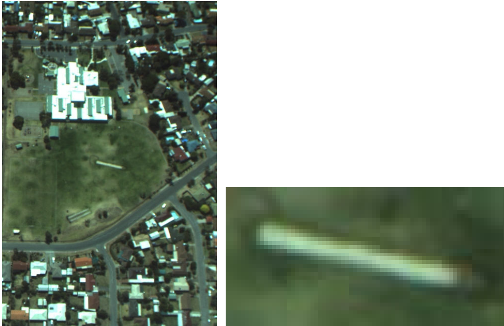
Figure 25 Frame 2200 showing cricket pitch used to test for band registration (facing east).
