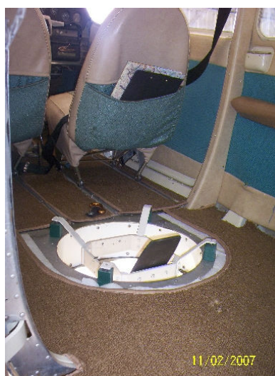
Figure 5 Camera port with mounting bracket attached, internal view.
