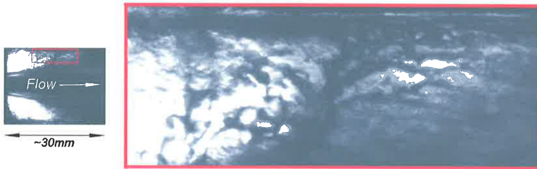
Figure 5.5 Condensed water at chamber perimeter during combustor operation at approximately time t \sim 0.7 seconds after ignition. P_{ch} \sim 45 bar.
