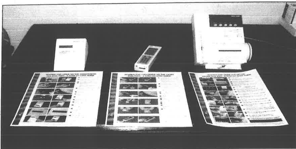
The point-of-care instruments being used at Port Lincoln: Cholestech lipid analyser (left) and the Bayer DCA 2000 (right). The instrument in the middle is the Abbott i-STAT analyser, another POC instrument that may be used at Port Lincoln in the future. Pictured in front of each instrument is a step-by-step guide that shows how to perform a test on each instrument. These guides were produced by the Flinders team as an educational resource to assist the PLAHS health workers.
