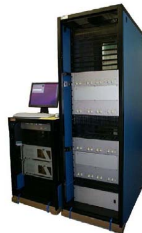
Figure 27 MF SA radar at Pontianak (left); 64 kW MF radar equipment (right)
