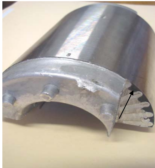
Figure 1.7: Photograph of a rotor with broken bars
