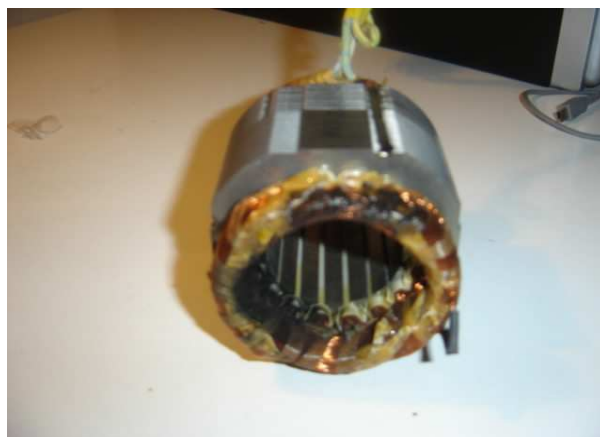
Figure 6.1: View of stator winding showing effect of shorted turns in early stages.
