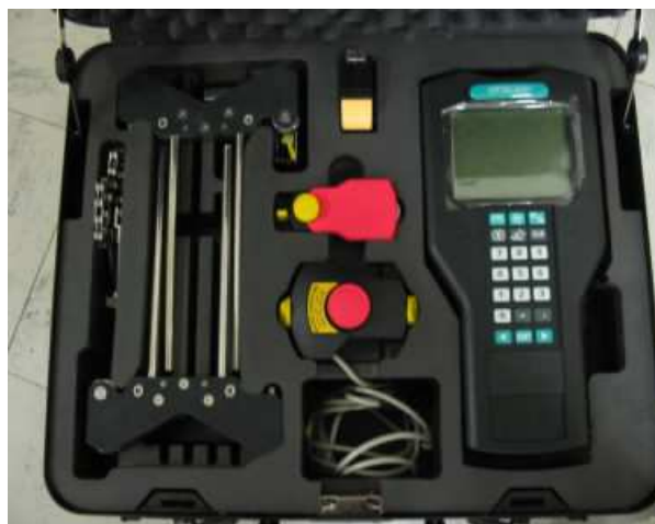
Figure 3.4: Laser Alignment Device used for precision alignment.
