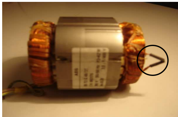
Figure 6.2: View of shorted turns in stator winding of faulty motor with.
