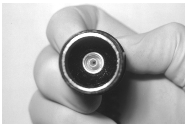
FIGURE 2a: Braun luer lock injection site tightly wedged in black endotracheal tube connector.
