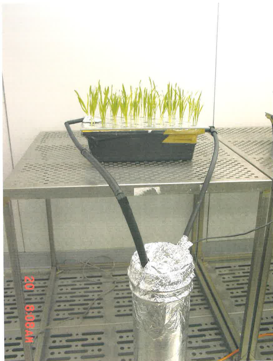
Plate 8.1. Hydroponic apparatus used to investigate the effect of Na exclusion on the uptake of other elements in Na excluding and non-excluding lines derived from the cross (Kalka#4*Na49).
