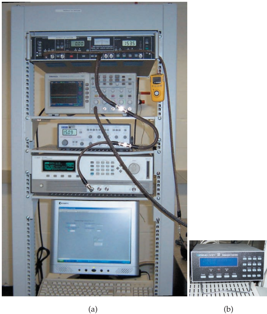
Figure D.8. Photograph of right part of the experimental apparatus shown in Fig. D.6. (a) Equipment in the instrument rack from top to bottom is as follows: an EG&G 5210 lock-in amplifier, a Tektronix TDS2014 digital oscilloscope, a TTI TG230 function generator, and an Agilent 8114 A high power pulse generator. (b) A CryoCon model 32 temperature controller, affording two-channel controller designed for fixed cryogenic applications.
