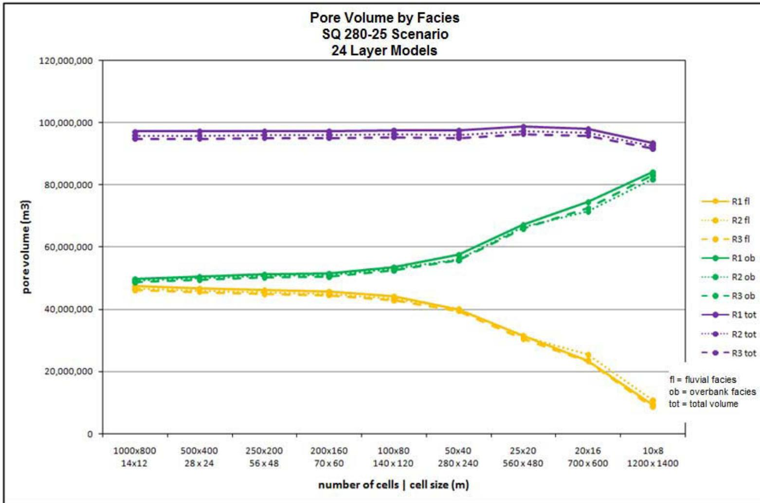
Figure 5.33. Pore volume by facies (fl: fluvial, ob: overbank, tot: total pore volume). 24 layers, SQ 280-25 scenario. Three realizations have very similar pore volumes associated with each facies for every grid design.
