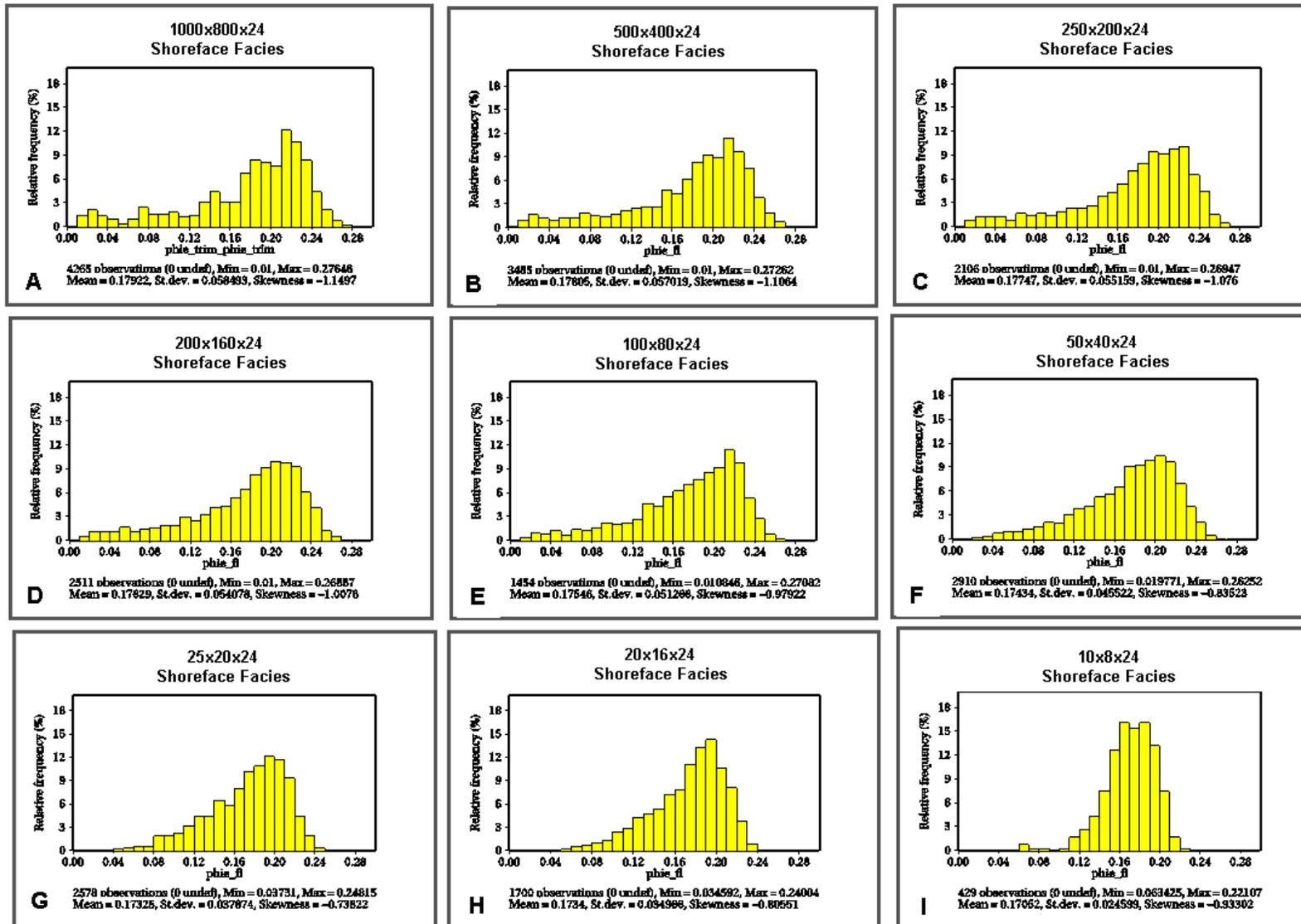
**Figure 5.31. SQ coast scenario - Shoreface facies porosity distribution.** The distribution of porosity values in the shoreface facies remains lognormal for all upscaled grids except the last (I).
