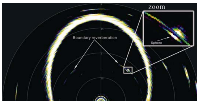
Fig. 4-9: Image when object echoes and reverberation are observed at the same range.
