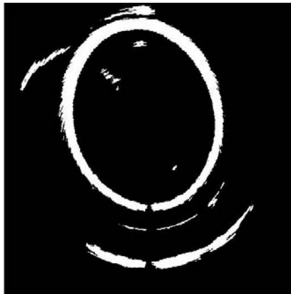
Fig. 4-16: Binary image after Otsu thresholding.
