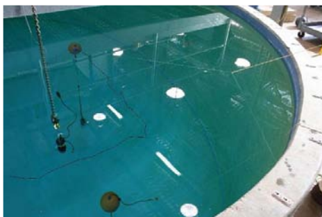
Fig. 4-35: Targets in the tank. The black line is the trajectory of the dynamic target. (The path is generated from a sequence of digital images by connecting the gravity centres together.)
