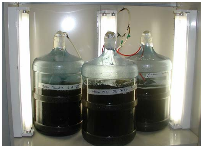
Figure 3.1 Photo-bioreactor carboys used to grow Pleurochrysis carterae
