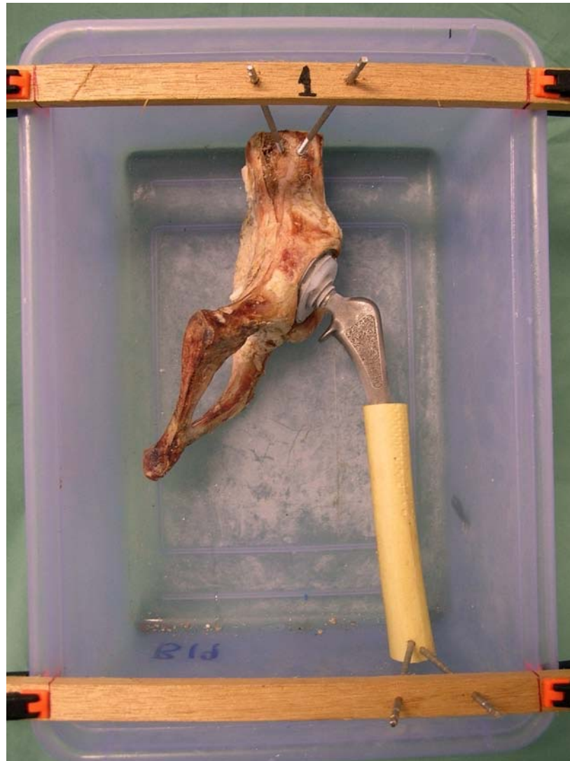
Fig.4.1 Photograph showing bovine acetabulum specimen model of total hip replacement positioned in a plastic container. The femoral component is inserted in to a plastic tube for additional stability. The specimen is fixed proximally and distally by Steinman pins to wooden plates and then clamped to the container.
