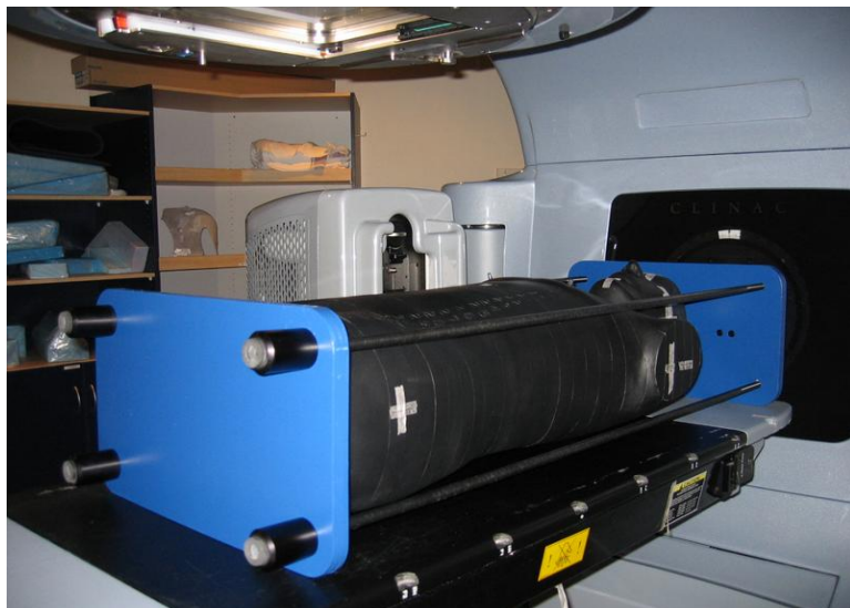
Figure 7.3. The TLD-loaded Rando phantom is placed on the treatment couch of the Varian iX linear accelerator. The laser beams were used to set up the phantom on the couch using the coordinates marked on the phantom for pelvic irradiation.
