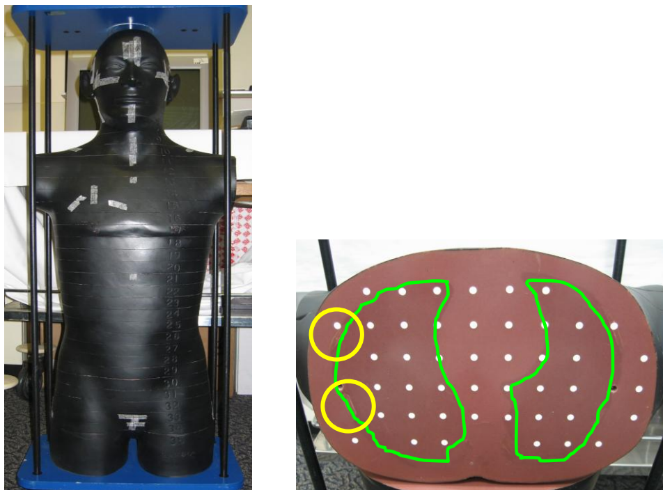
Figure 7.1. (Left) The anthropomorphic Rando phantom consisting of 35 section slices. The phantom sections are individually numbered and all sections are assembled in the clamping device.
