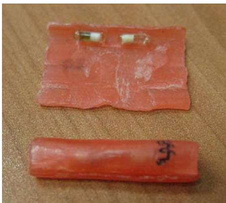
Figure 7.2. A picture shows a TLD plug made from the tissue equivalent wax and a pair of {}^6\text{LiF:Mg,Cu,P} and {}^7\text{LiF:Mg,Cu,P} TLD rods. A permanent ink marking pen is used to mark the number of the TLD plug.
