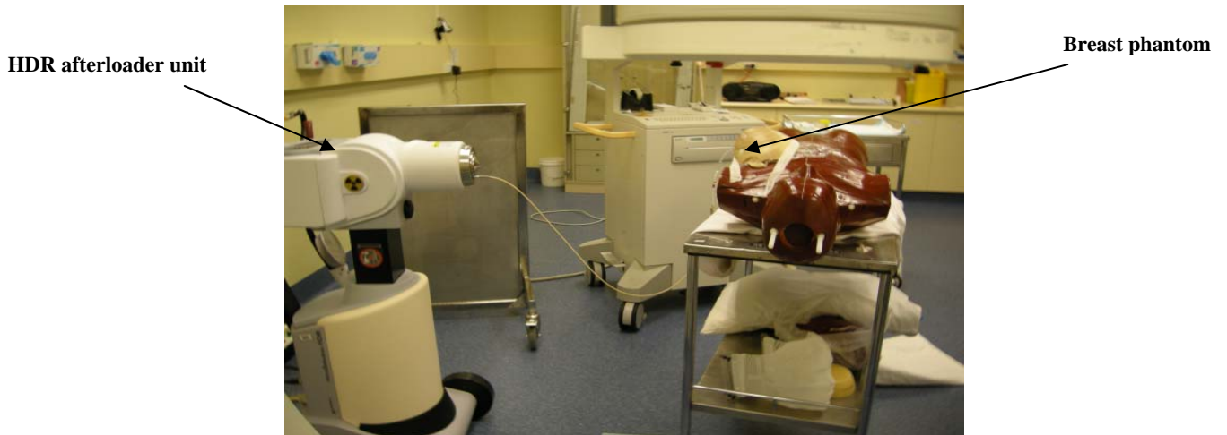
Figure 5.15. Experimental setup for dose measurements in the breast phantom using TLD chips.
