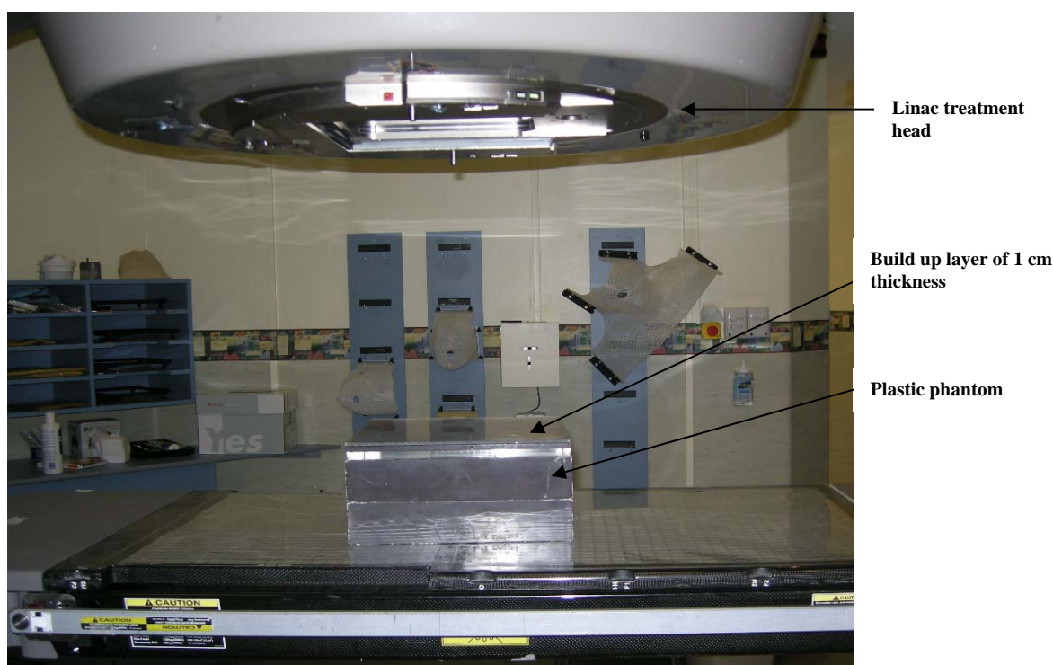
Figure 5.13. Experimental setup for the measurement of the sensitivity correction factor of the LiF TLD-100 chips.
