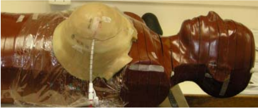
Figure 5.3. The inflated balloon placed inside a designed breast tissue equivalent phantom which is attached to the Rando ® anthropomorphic phantom.
