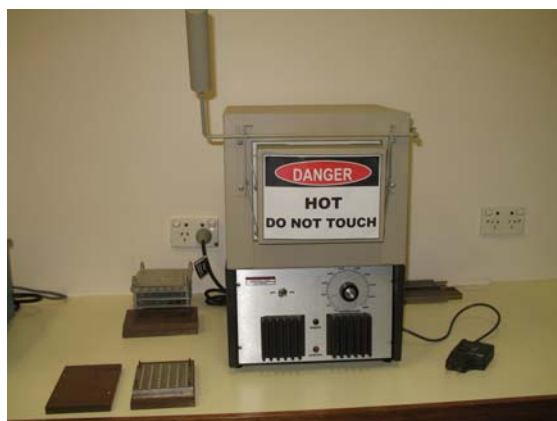
Figure 5.10. Oven and aluminium blocks that were used for annealing and cooling of TLDs respectively.
