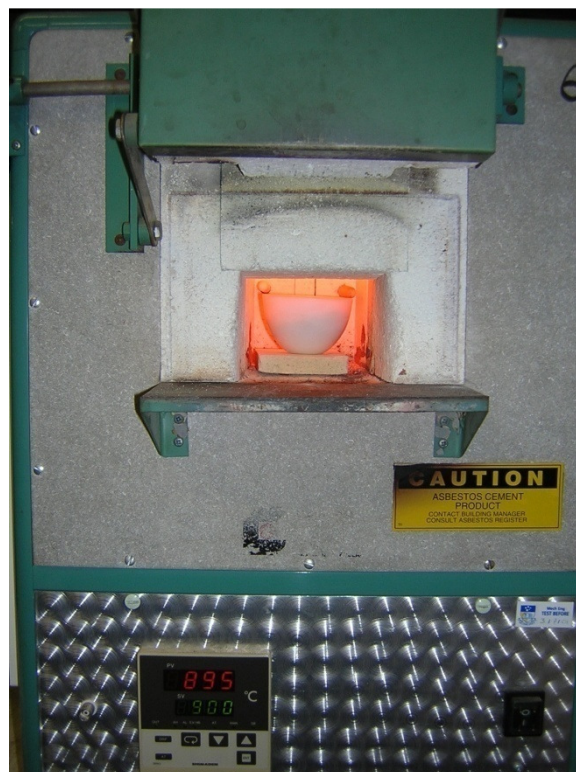
Figure 6-1: Photo of the crucible bowl inside the preheated muffle furnace.
