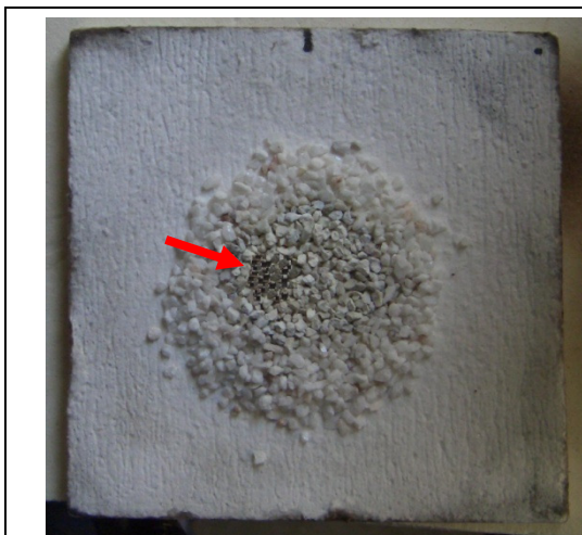
Figure D-5: Photo of d_c = 2.855\text{mm} diameter marble spread over refractory board to form 80mm \varnothing circle, after calcination.
