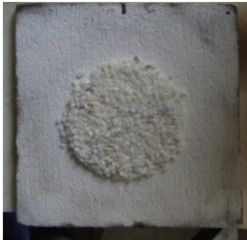
Figure D-1: Photo of d_c = 2.855\text{mm} marble spread over refractory board to form 80mm diameter circle, before calcination.
