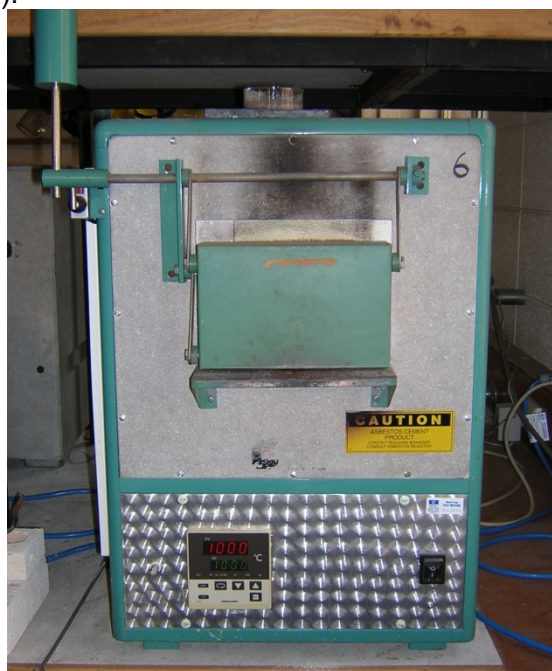
Figure 4-2: a). Photo of the electric Carbolite muffle furnace used for the muffle furnace experiments. b). schematic showing location of the temperature measurement points within the muffle furnace.
