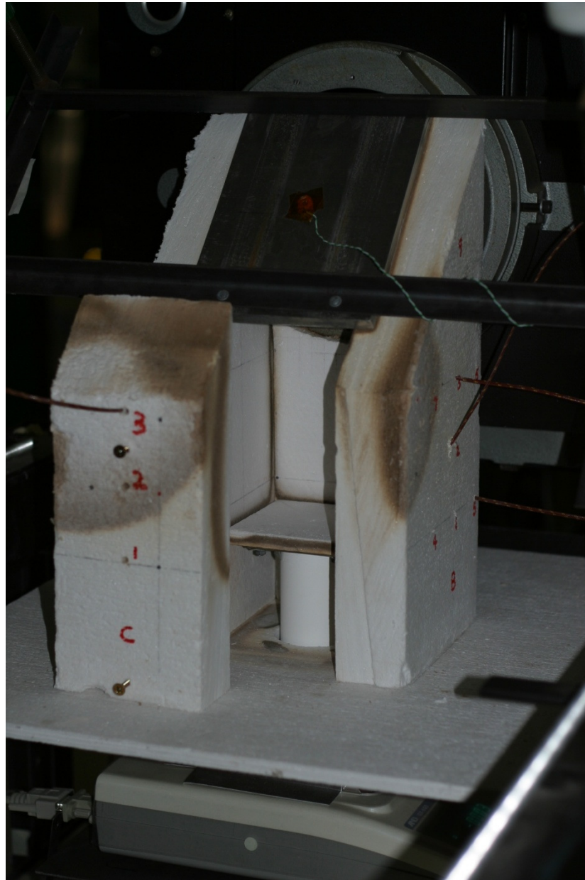
Figure 4-14: Photograph of the solar furnace with the rear wall removed, showing the calcination platform system.
