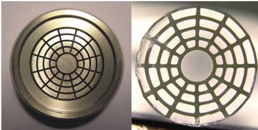
FIGURE 5.8: Preform 3. Left: Photograph of the exit-face of the stainless-steel die used to extrude a 5 cm diameter lead-silicate (F2) glass billet to create the third air-Bragg fibre preform. Right: Photograph of the end of the produced preform (cleaved). The diameter of this section of the preform is about 6 mm.
