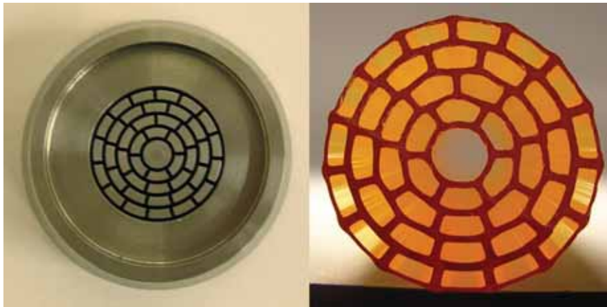
FIGURE 5.5: Preform 2. Left: Photograph of the exit-face of the stainless-steel die used to extrude a 5 cm diameter bismuth-oxide glass billet to create the second air-Bragg fibre preform. Right: Photograph of the end of the produced preform (sawed flat). The diameter of this section of the preform is about 2 cm.
