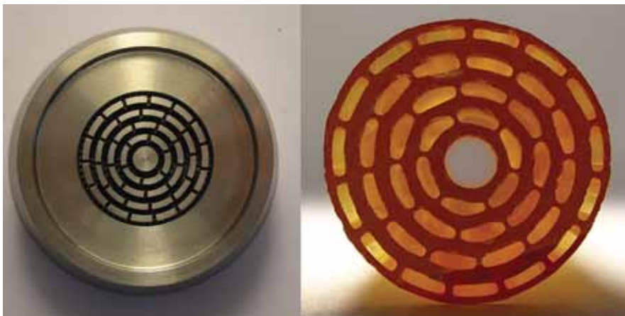
FIGURE 5.4: Preform 1. Left: Photograph of the exit-face of the stainless-steel die used to extrude a 5 cm diameter bismuth-oxide glass billet to create the initial air-Bragg fibre preform. Right: Photograph of the end of the produced preform (a glass-cutting saw has been used to produce a clean, flat, end-face). The diameter of this section of the preform is about 2 cm.
