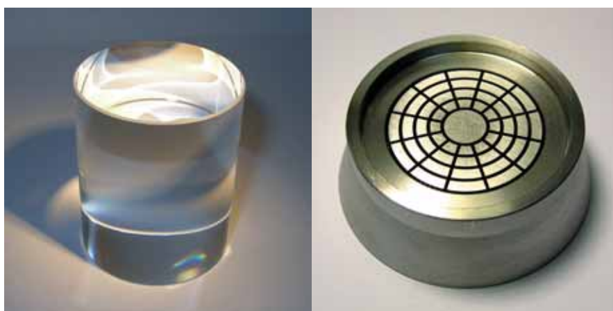
FIGURE 5.1: Left : a 5 cm diameter soft-glass (lead-silicate, F2) billet. Right : the exit-face of a spider-web structure stainless-steel extrusion die used for soft-glass preform fabrication (same as in Fig. 5.8). Like this die, all dies made to extrude glass billets of diameter 5 cm shown here have an exit-face outer rim diameter of about 44 mm and entrance diameter of about 5 cm.
