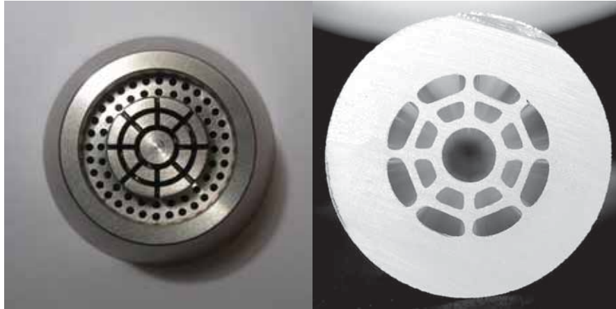
FIGURE 5.13: Preform 4. Left: Photograph of the exit-face of the stainless-steel die used to extrude a 3 cm diameter lead-silicate (F2) glass billet creating a 2-Ring air-Bragg fibre preform with colinear struts and a thick outer jacket . The exit-face outer rim diameter is about 23 mm. Right: The fabricated preform.
