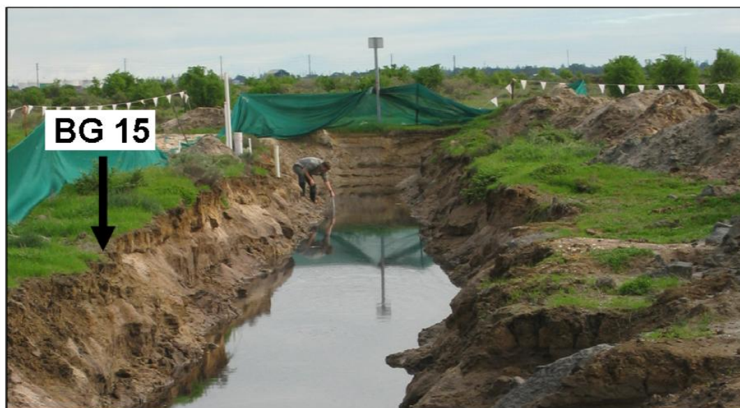
Figure 8-22 Photo (winter 2003) of the drain transecting sulfuric and sulfidic materials at Gillman Focus area A. Soil profile BG 15 is located on the left (western) wall of the drain. The drain was excavated in August 2002 as part of a lime slot remediation trial. The water in the drain had a pH that ranged between 2 and 3. Salt efflorescences (with pH values ranging from 0.8 to 3) precipitated on drain walls, particularly during summer months and were washed away after heavy rains. The drain runs north-west, positioning profile BG 15 in direct sunlight for the greater portion of the day.
