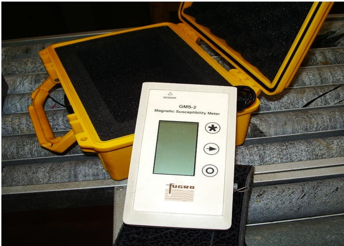
Figure 4.8: A Magnetic Susceptibility Metre model Digital Fugro GMS-2.
