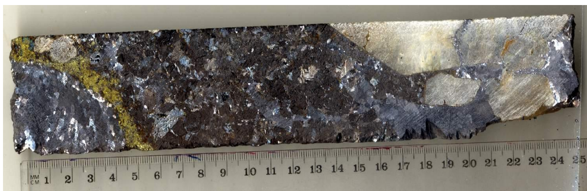
Figure 2.3: Coarse sulphide minerals including galena (grey), sphalerite (black), chalcopyrite (yellow) and white quartz in a cataclastic massive sulphide rock of the Western Mineralisation (drill hole 4033 at 353.2 m). The structural position of cataclastic ore is unknown and may well remain so until further underground mining commences.
