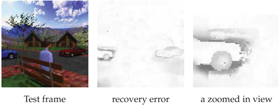
Figure 5.1. The results of the local computation weighted by \omega_{intensity}^{(k)} \cdot \omega_{occlusion}^{(k)} \cdot \omega_{residual}^{(k)} \cdot \omega_{consistency}^{(k)} . The motion boundary between the blue car and the background is over-smoothed. Darker intensity indicates larger errors.
