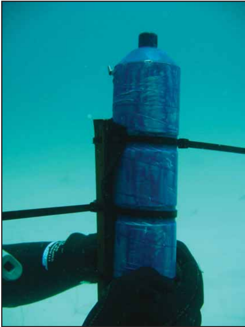
Mooring a Vemco™ VR2W acoustic receiver. Photo credit: Simon Bryars.
