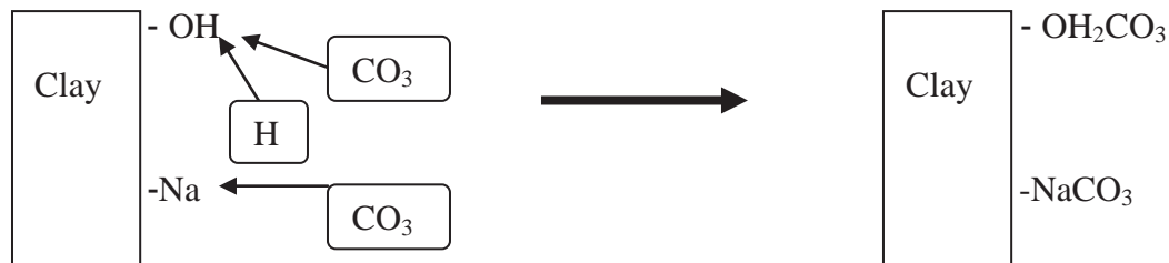
Figure 5.1 Mechanism for the sorption of carbonate to clay particles.
