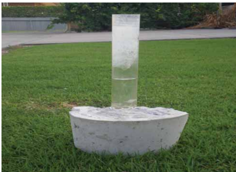
Figure 6.3: Photo of the sediment trap used for the experimental study of sedimentation process within Cox Creek wetland. Note that each cylinder was placed at the inlet and outlet of both Reed Bed and Pond 1.
