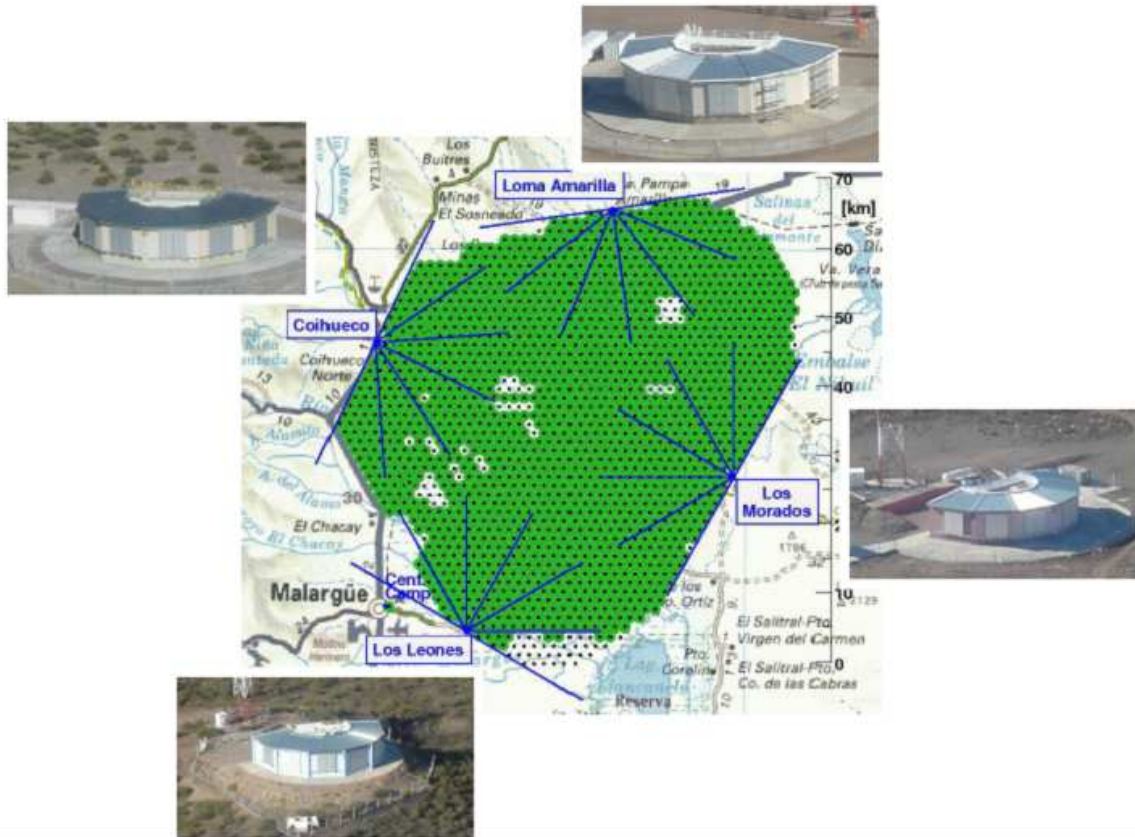
Figure 4.1.: A map of the Pierre Auger Observatory in Argentina. Each water Cherenkov tank is represented by a black dot. The array is surrounded by the four fluorescence stations as shown. The fields of view of the 24 telescopes are indicated by the blue lines.
