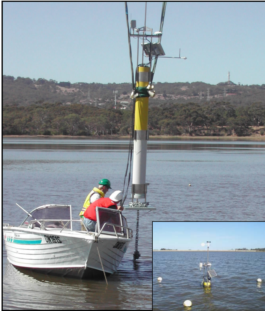
Figure 63 A spar-buoy supporting three separate thermistor strings having different anchoring arrangements to allow stratification monitoring in the epilimnion (surface layer), metalimnion (thermocline layer) and hypolimnion (bottom layer) of a reservoir, no matter how the water level changes. The perforated plate at the bottom of the buoy acts as a hydraulic damper to prevent the buoy 'bobbing' in rough water. The length of the chain wrapped around this damper plate is adjusted to change the flotation depth of the spar buoy, which sits low in the water (bottom, right) to allow correct operation of the net radiometer. The latter is part of the weather station cluster mounted on the buoy to monitor wind and solar energy. The station uses cellular phone long-haul telemetry and VHF ship-to-shore SCADA radio systems.
