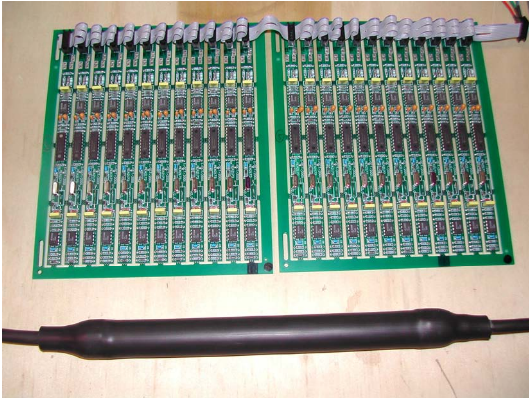
Figure 19 Twenty-four sensor circuit boards are shown before being broken-out from the PCB panel form in which they are manufactured. They are shown linked by ribbon cable (top) to power, program and test them prior to encapsulation. They are then potted inside a threaded PVC tube with a cable-gland and O-ring at each end. A heavy-walled adhesive heatshrink is then shrunk over the whole assembly to form a third level of waterproofing (bottom).
