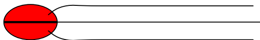
Figure 29 A thermilinear thermistor, consisting of a high-resistance thermistor thermally and electrically bonded to a low-resistance thermistor.
