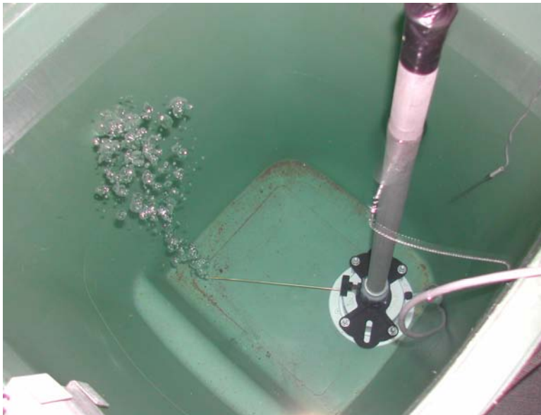
Figure 42 The standpipe is shown in the water column, with the electronics below and the Hagen-Poiseuille flow control pipe to the left (the latter was later replaced by 33 m of wound plastic pipe to lower the Reynolds Number below turbulent flow speeds). Rather than step-change height, the method shown here purged the vertical standpipe using compressed air. Uncapping the top of the standpipe allowed water to flow back in with a first-order time-constant.
