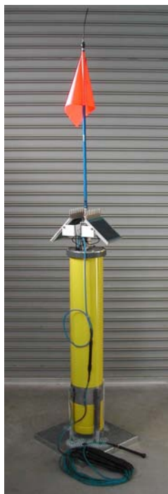
Figure 61 A radio-linked ship-to-shore buoy supporting a SDI-12 thermistor string. No data logging occurs on the buoy; instead, all data is transmitted immediately after each 15-minute measurement.
