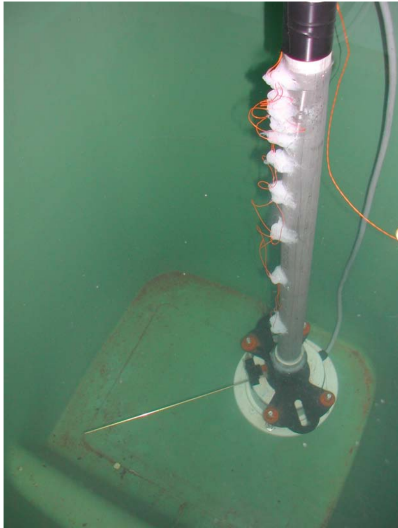
Figure 43 The seepage meter standpipe is shown with the ‘level sensing’ thermistors arranged in a logarithmic spacing up through its height. The level sensor spacings were chosen to allow roughly equal time intervals for the arrival of the water-air front at each heated sensor as the water level rose up through the column with decaying velocity, flowing in from the main tank through the flow control pipe on the left.
