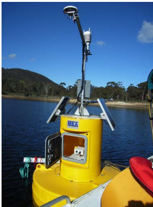
Figure 62 This Sealite buoy supports a full logging system, an integrated weather station capsule (Vaisala WXT-510) for air temperature, relative humidity, (drum-head) rainfall sensor, barometric pressure, ultrasonic wind speed and direction and separate global solar and net radiation sensors. All of these sensors are SDI-12 compatible, as is the electronic compass (seen through the instrument door) developed to give a local reference direction for the wind direction sensor. The data logger reads only SDI-12 sensors, and includes Next-G cellular-phone telemetry for remote data collection.
