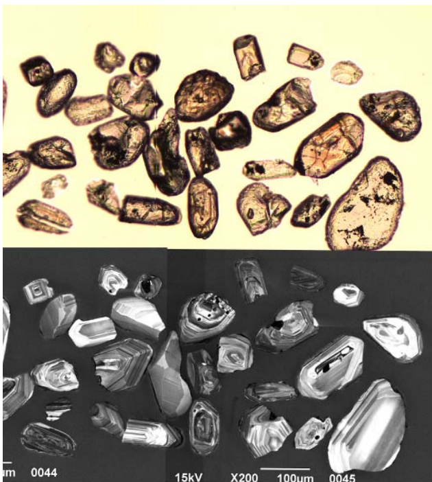
Figure A.16. Selected transmitted light (top) and cathodoluminescence (bottom) images of zircon grains from the Kuridala siltstone (Mount Angelay and Malbon, 1976838).
