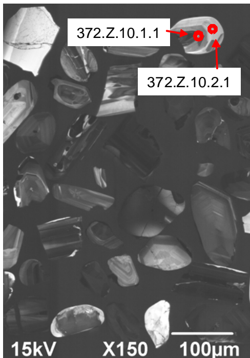
Fig. A.9. Cathodoluminescence images of zircon grains from the volcanic rock within the Candlow Formation (North Head, 1999372). Analysis with sample numbers; 372.Z.10.1.1 & 372.Z.10.2.1 consisting of low ^{232}\text{Th}/^{238}\text{U} values (Fig. A.10) are interpreted as zircon recrystallisation (Table A.2, see Hoskin and Black (2000) for more details).
