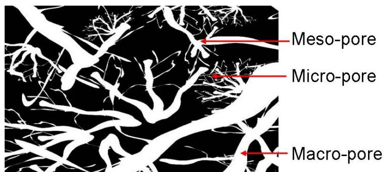
Figure 5-20 Illustration of three types of pore structure in char particles, namely micro-, meso- and macro-pores; a radius less than 1 nm is defined as micro-pores and between 1 ~ 25 nm and greater than 25 nm are defined as meso- and macro-pores, respectively.
