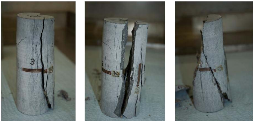
Figure 3.13: Failure pattern of core aggregate cylinders.
