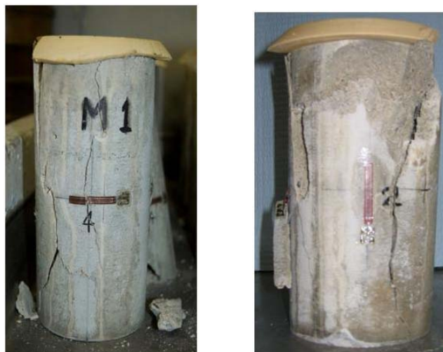
Figure 3.10: Failure pattern for mortar cylinders
