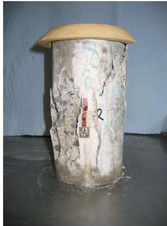
Figure 3.7: Failure pattern of concrete cylinder
