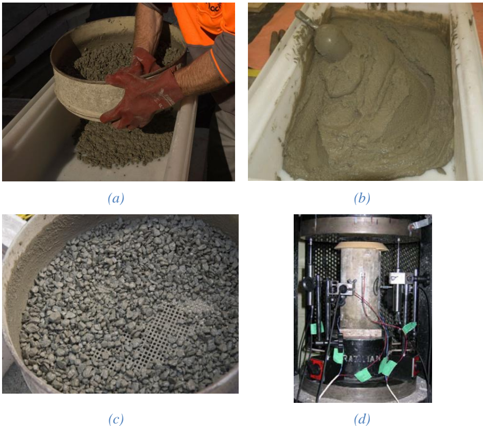
Figure 3.3: (a) how to produce the mortar; (b) fresh mortar; (c) separate aggregate; (d) 100mm×200mm mortar cylinder
