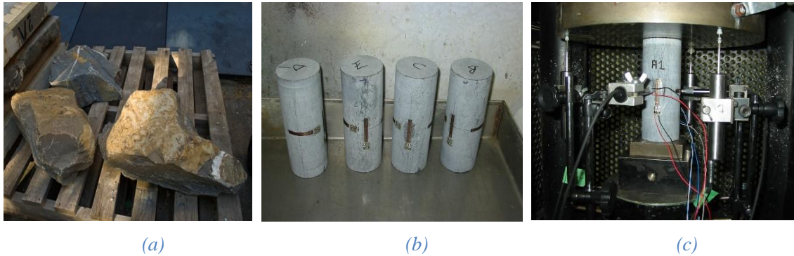
Figure 3.4: (a) rock sample; (b) 58mm diameter and 150mm length core aggregate cylinder; (c) aggregate test set up
