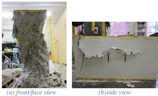
Figure 4.22: Failure mode of concrete test Test(II)6-125×250×500
