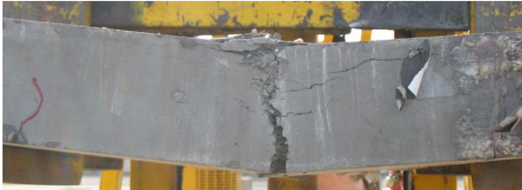
Fig. 1 Compression wedge in a beam [2]
