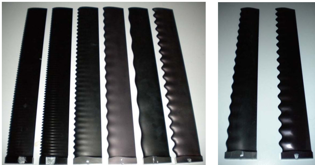
Figure 3.4 – Set of NACA 0021 and NACA 65-021 airfoils with tubercles (left and right respectively).
