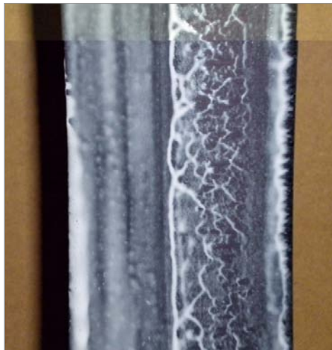
Figure C3 – Surface flow visualisation of mid-span using toothpaste ( \alpha = 10^\circ , U_\infty = 25\text{m/s} )
