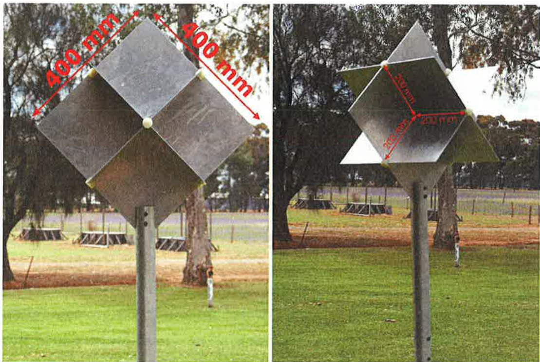
Figure 6-26 Cluster corner reflector
