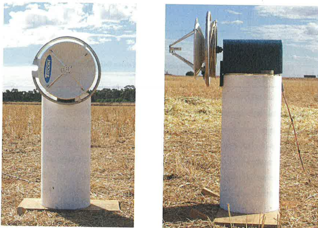
Figure 3-43 Rotating delay line calibrator
