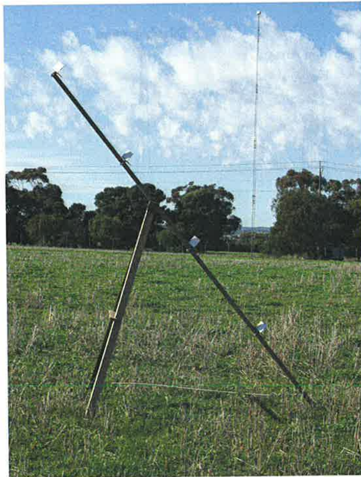
Figure 3-26 Trihedral corner reflector array
