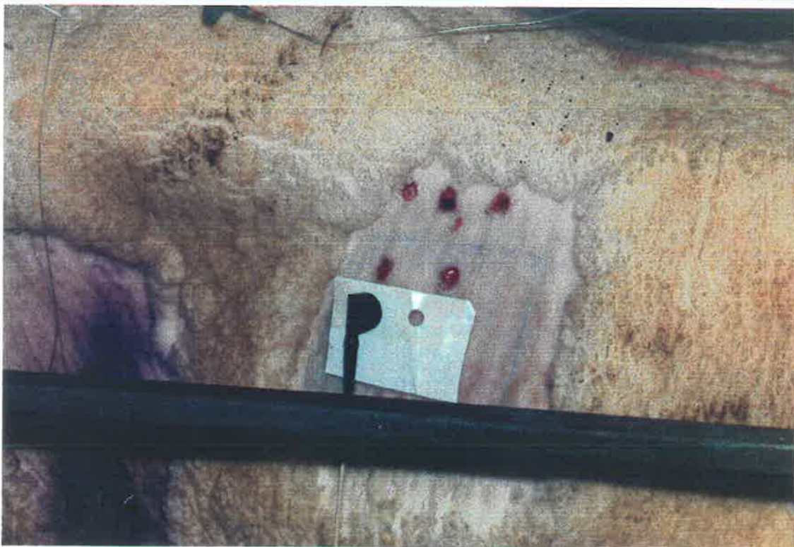
Plate 3.1. Photograph of the laser Doppler velocimeter probe placed within the midside tattoo patch of a sheep. The probe is attached to the skin with adhesive tape topped with double-sided sticky tape.
