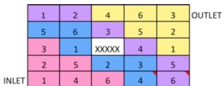
Figure 25: Schematic diagram of tooth root sample positioning. The flow cell inlet is in the lower left and the outlet in the upper right. The flow cell was divided into 4 zones (Zone A, B, C and D, shown as pink, Blue, purple and yellow, respectively). The numbers represent each of the six treatment groups so each treatment group contained one tooth root from each zone.
