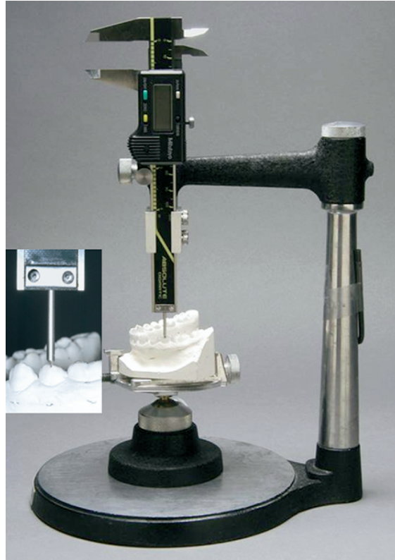
Figure 4.6. Digital calipers vertically mounted on a dental surveyor used to measure the maximum depth on leveled study models as described in Figure 4.5. (Marshall et al. 2008).
