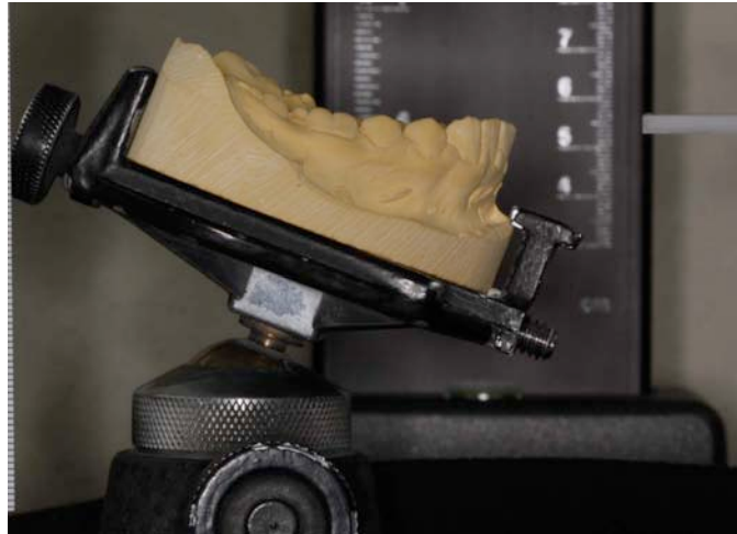
Figure 7.4. Mounted model with standardised occlusal plane, the figure illustrates the ability of the study model occlusal plane to be adjusted 360°.
