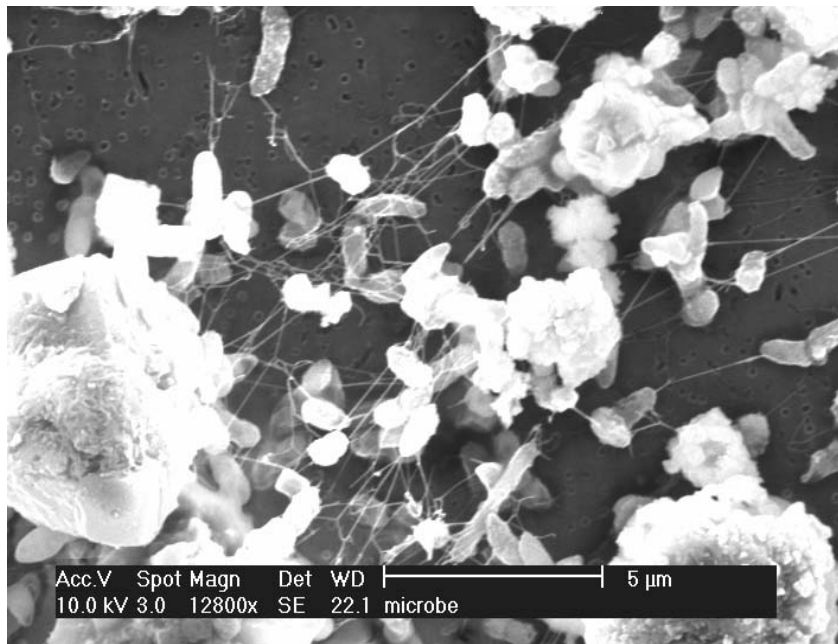
Figure 4-4 SEM images of bacteria and their microfibrils forming aggregates
