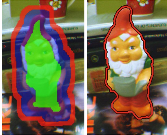
Figure 6.5: The graph cut region and resulting silhouette. The cut is performed on pixels within the blue region, with pixels in the red region labelled as background, and pixels in the green region labelled as foreground
