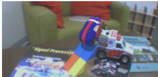
Figure 6.4: A synthetic car model casting a shadow onto a real ramp and toy ambulance
