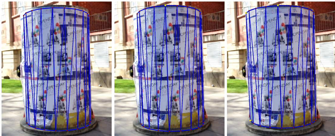
Figure 3.13: Manually refining the fit for the cylinder model. On the left, the initial fitting result. In the centre, the fitting result with one vertex specified. On the right, the fitting result with three specified vertices.
