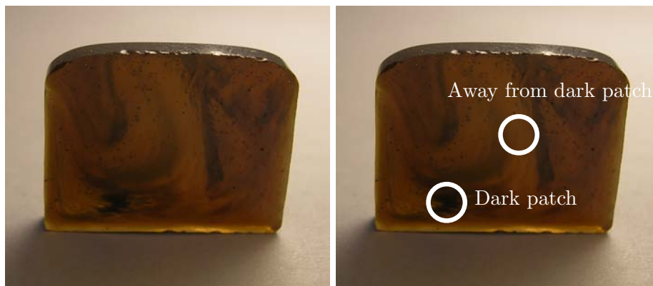
FIGURE 3.5: Sample slice of glass G1. The glass is dark due to a high concentration of added diamond (compare to e.g. G3 in Section 3.4.3). The dark swirls suggest an inhomogeneous mixing. (Right) Same image labelled with an area characteristic of a ‘dark’ patch and away from these patches.
