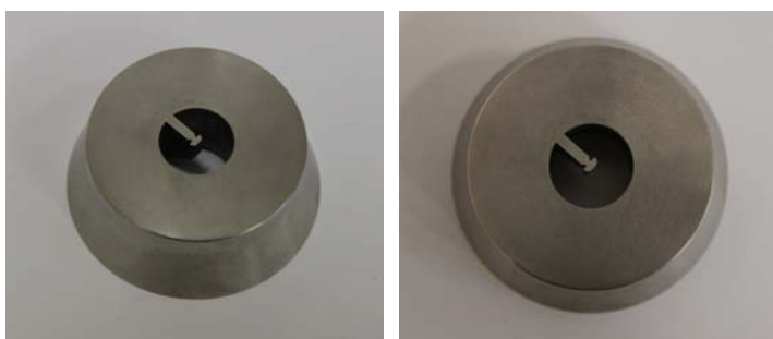
FIGURE 4.9: Images of the extrusion die used for the outer tube preform T6b.
