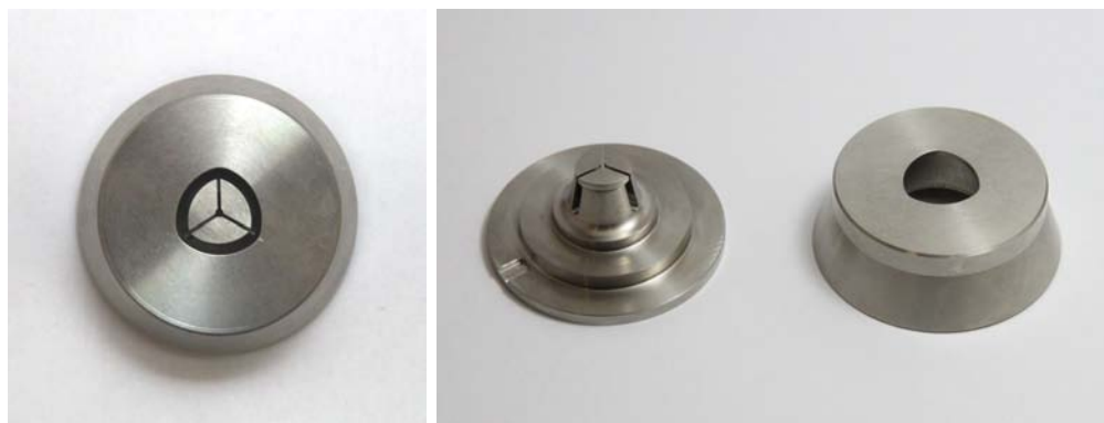
FIGURE 4.2: Die design used to fabricate a wagon-wheel preform.
