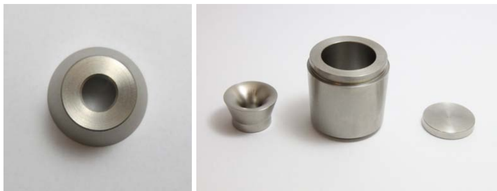
FIGURE 3.1: (Left) Die design used to fabricate a rod preform. (Right) Die shown with the sleeve that holds the cylindrical glass billet and the plate to which the ram applies force.
