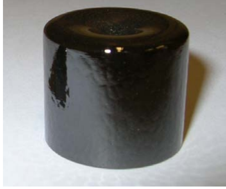
FIGURE 3.11: Sample G2, doped with non-irradiated NV . The dark appearance is attributed to the high diamond concentration, as for sample G1 above (see Section 3.4.1).
