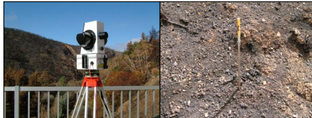
Above: (L) Maptek I-Site 4400LR terrestrial laser scanner (R) Erosion pin Below: Modelled surface representing volume change between Feb 07 and May 07 based on a 1m signed surface difference. Inserts are photos from field site.
