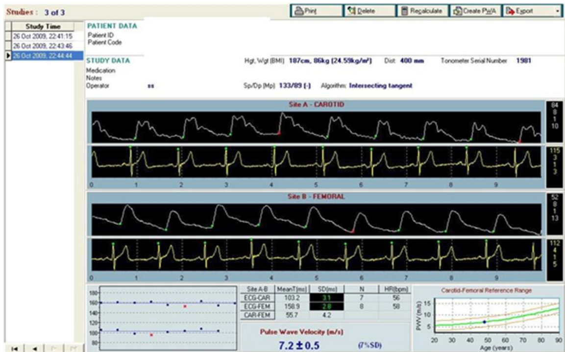
Figure 2.4: Screen shot of PWV analysis post measurement, showing carotid and femoral pressure wave traces, timed to cardiac rhythm strip. PWV, in m/s, shown at bottom of the screen, with reference range corrected for age in the bottom right corner.
