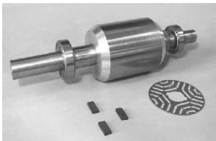
Figure 2.22: Multiple-barrier rotor with rare-earth magnets
