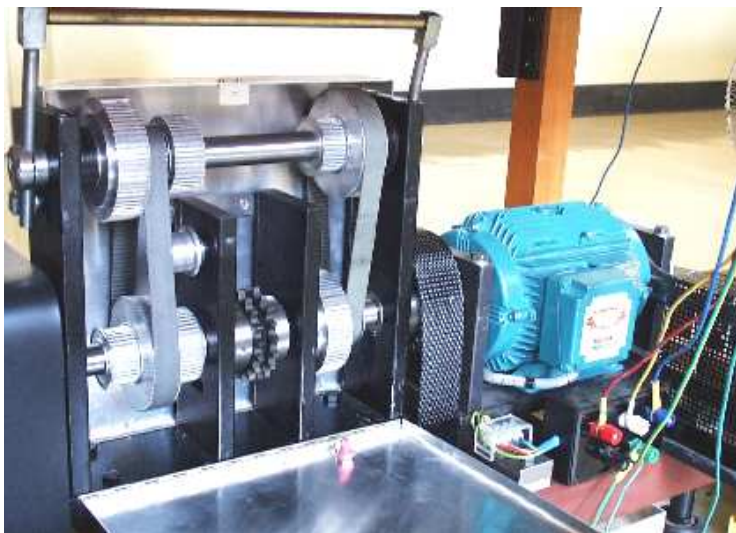
Figure 2.25: Variable gearbox for the dynamometer rig
