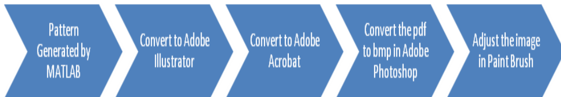
Figure 4-2: Workflow adopted to import actual geometry from MATLAB to MS Paintbrush
