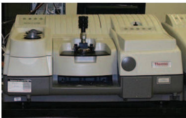
Figure B.1. Thermo Scientific Nicolet 6700 FTIR system. The FTIR system used for the baby milk powder measurements. The centre of the system contains the press to push samples down onto the measurement window.
