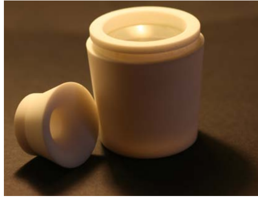
Figure 112: Rod die and sleeve fabricated from MACOR, with FK5 billet shown inside the sleeve.
