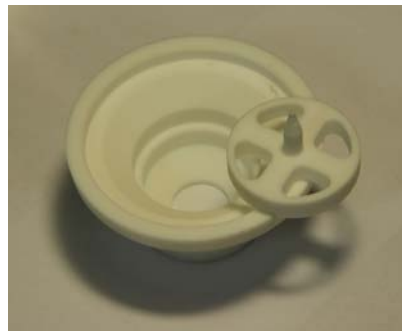
(d) Cross-type die for 10 mm outer 1 mm inner diameter tube extrusion. This die design as been shown in the past to reduce the required force with identical extrusion parameters.
