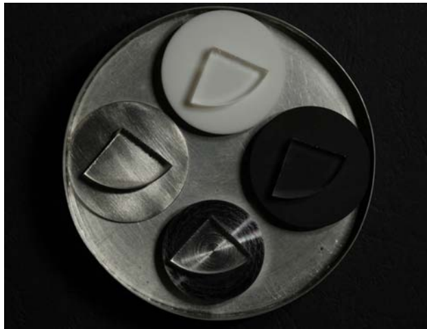
Figure 125: Die materials trial on platinum plate, with polished FK5 wedge on each disk. From top, clockwise - MACOR, graphite, Inconel, stainless-steel.
