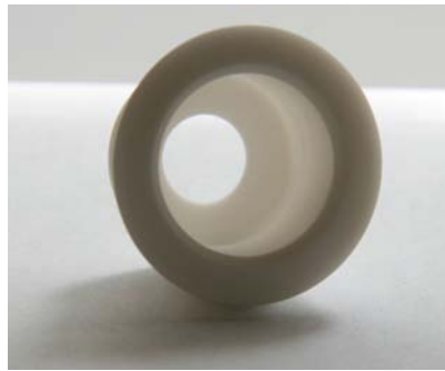
(b) MACOR tube die outer assembly, iteration 1. A standard tube-die inner was also fabricated from MACOR, however this is not shown here.
