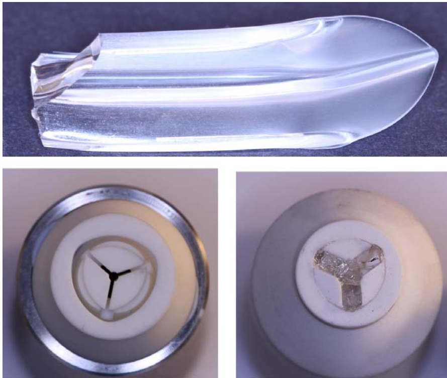
Figure 119: (top) Extruded FK5 wagon-wheel preform. The location of the preform where the die failed can be seen where the outer section of the struts rapidly expands. (bottom left) MACOR wagon-wheel die before extrusion. Note the gap between the struts. (bottom right) MACOR wagon-wheel die after extrusion. The die has failed part way through the extrusion, pushing the die parts out and creating a “Y” shape.”
