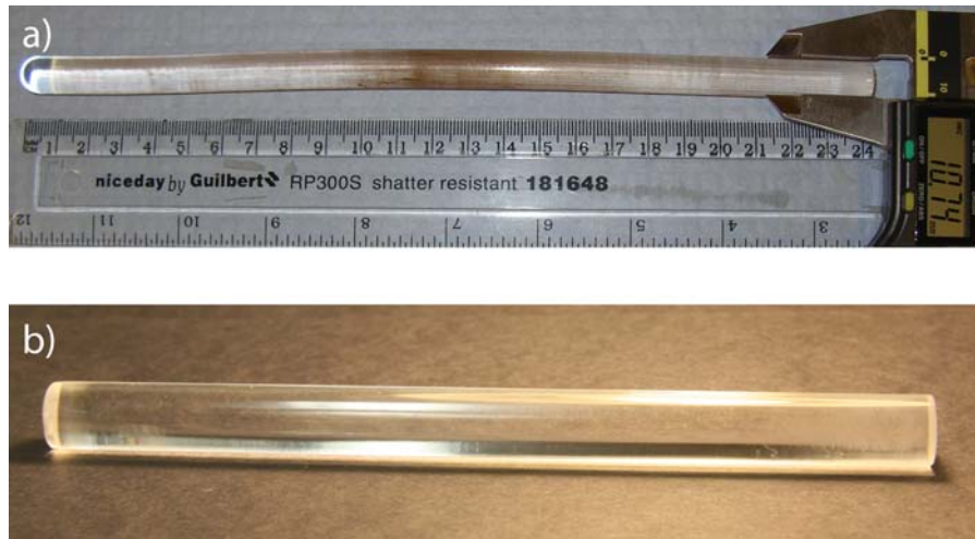
Figure 110: a) N-FK5 extrusion trial one. The surface has been significantly degraded, showing what appears to be rust along the length of the preform. b) N-FK5 extrusion trial one after the preform was cut, and the surface manually polished along its length.
