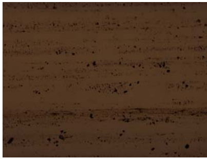
(a) N-FK5-1 extruded through stainless-steel die.
