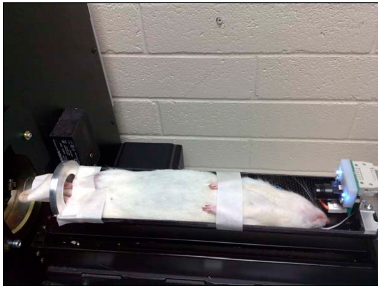
Figure 2. In vivo micro-CT imaging of rat hind limbs with the rat on the scanner bed in supine position.
