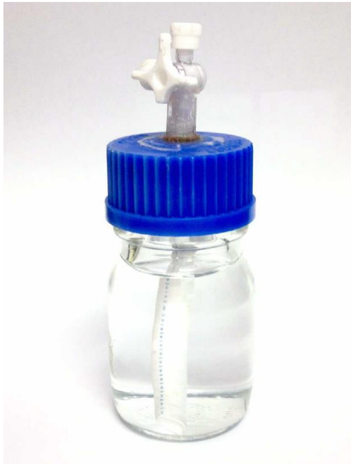
Figure 2.7: A vacuum container consisting of a 100 mL glass jar filled with 0.9% saline solution and a portion of PTFE. A BD Connecta™ three-way tap with luer-lock™ has been drilled and glued into the cap so air can be withdrawn from the jar using a syringe.
