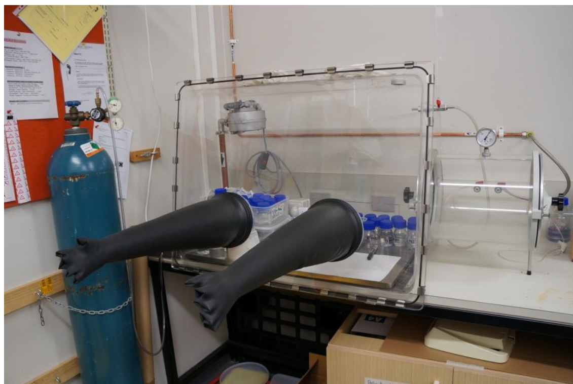
Figure 2.1 The argon-filled anoxic glove box used in this work.
