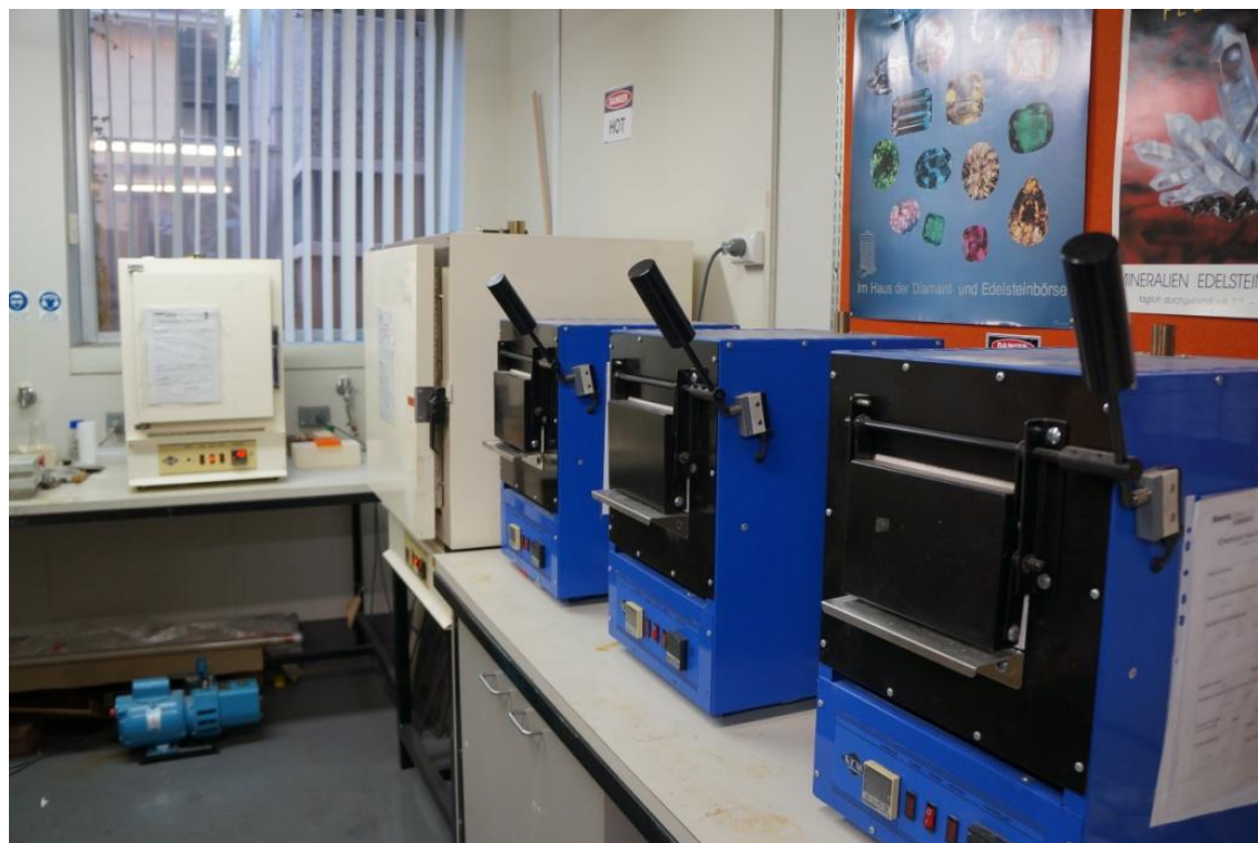
Figure 2.4 Muffle furnaces (blue) and ovens (creamy) used in this work. These furnaces/ovens are programmable and the temperature can be controlled precisely within \pm 2 °C. The maximum working temperatures of the furnaces and ovens are 1150 °C and 500 °C, respectively.
