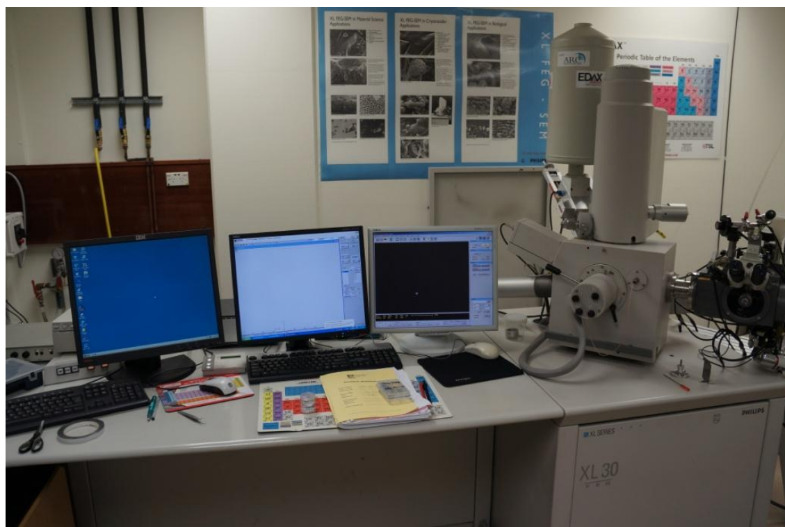
Figure 2.7 The Philips XL30 Field Emission Scanning Electron Microscope.
