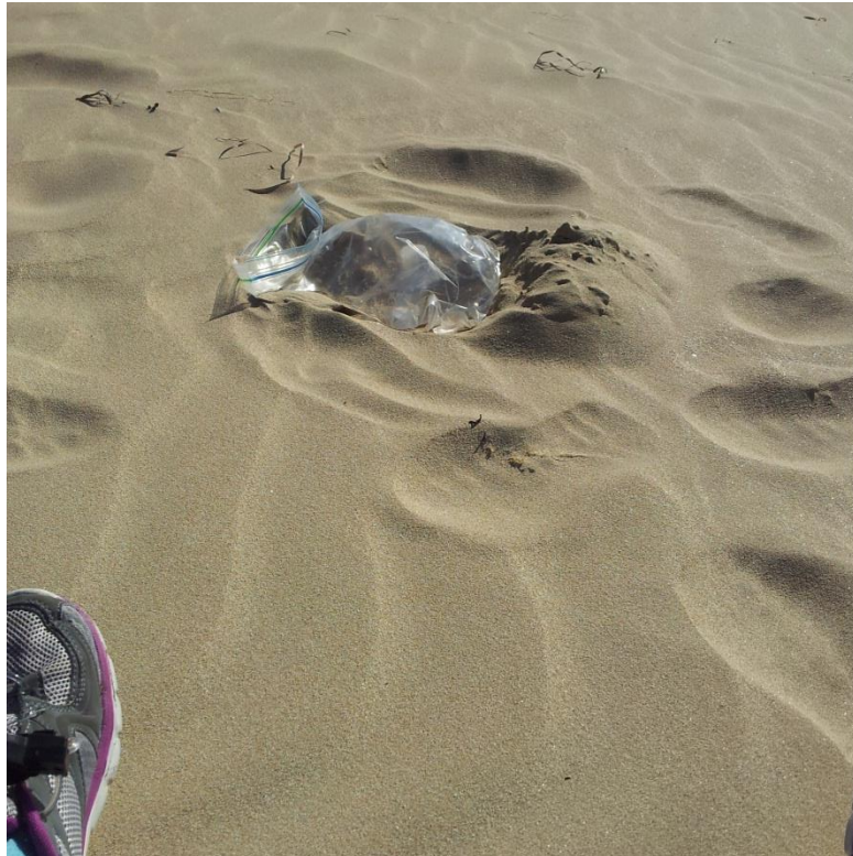
Figure 7.1: The 'sand trap' used to collect the sample. Wind was blowing sand from the left to the right of the picture.
