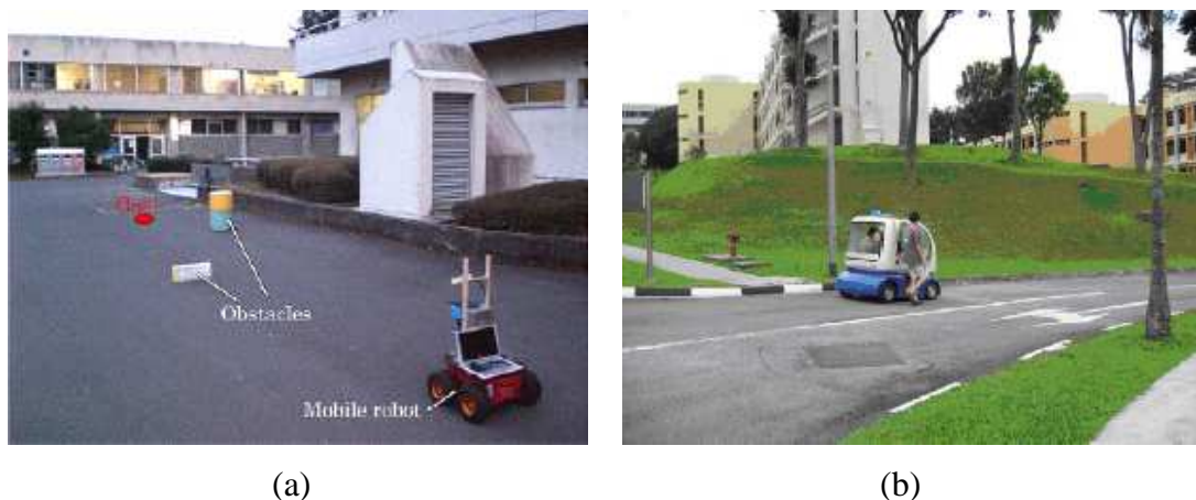
Figure 2.16 Outdoor navigation (a) Pioneer3-AT with URG and SICK (Chang et al. , 2009) (b) The Cycab used in the experimental works (Zhang et al. , 2006).
