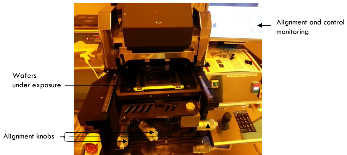
Figure 6.24. Lithography. Wafer under exposure, inside the lithography machine.
