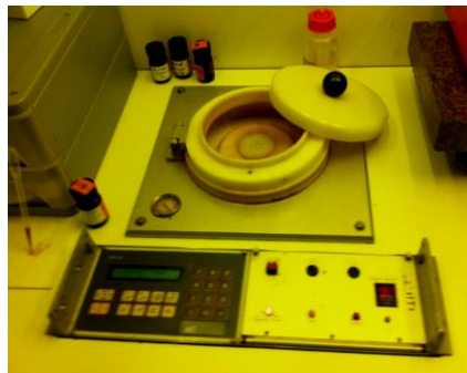
Figure 4.3. Spinning machine. By adjusting the speed to 3000 rpm and running it for 15 sec, the polyimide mixture on the surface was equally spread to about 0.3-0.4 \mu m thickness.
