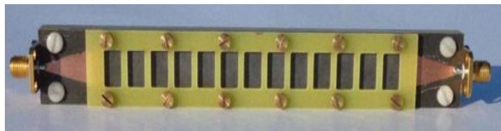
Figure 2.13. Leaky-wave tunable antenna. Fabricated liquid crystal tunable leaky wave antenna based on a composite right/left-handed waveguide structure, with beam steering capability. The maximum measured obtained beam tilt is \pm 10^\circ degree around broadside [16].
